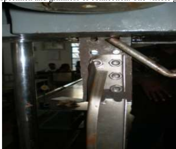
Figure 5 Block shear failure mode for single lipped angle specimen
