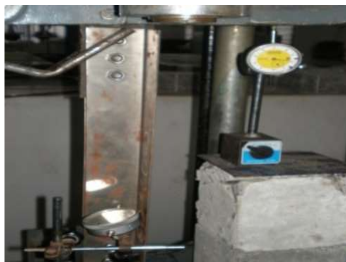
Figure. 2 Single plain angle connected to gusset plate
