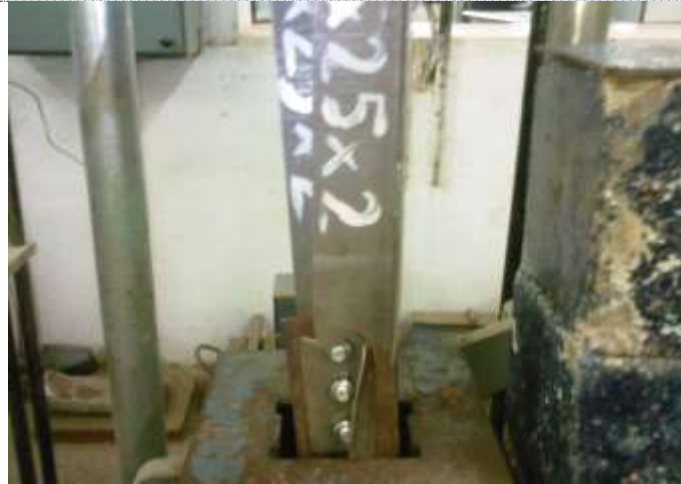
Figure 6. Net section failure mode for double plain angle specimen connected to opposite side of gusset plate
